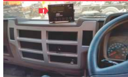
1. Reefer Temp Control Unit
