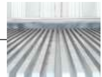
Aluminum T-Section on front panel & Floor for better air circulation and Drain Pipe for Easy Drainage
