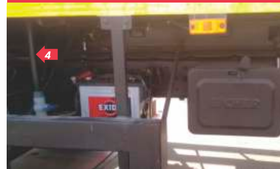
4. Drainage pipe for water accumulated in the reefer container
